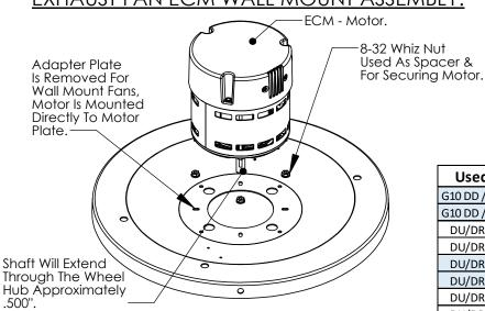
EC Motors on DU/DR 10 and 12 mount directly to the top plates without isolators or adapter plate.
