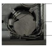
Nidec Motor Shown. Orientate the motor so the wiring is on the left side to minimize exposure to heat. Connect the motor wiring to the harness:
