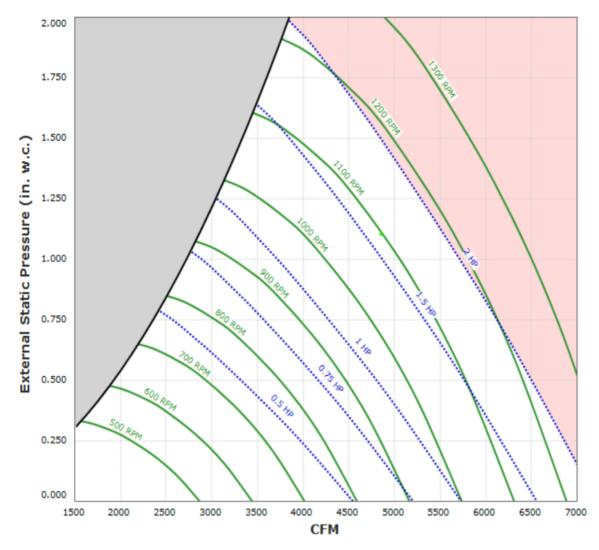
Max Sizable RPM= 1600 RPM. Curve shown extended beyond this point for reference only.
