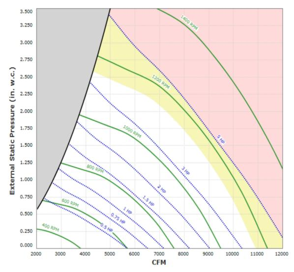
Max Sizable RPM= 1350 RPM. Curve shown extended beyond this point for reference only.
