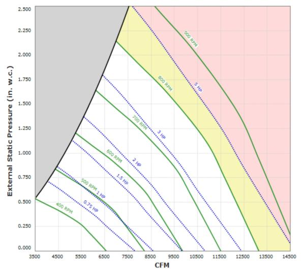
Max Sizable RPM= 1000 RPM. Curve shown extended beyond this point for reference only.
