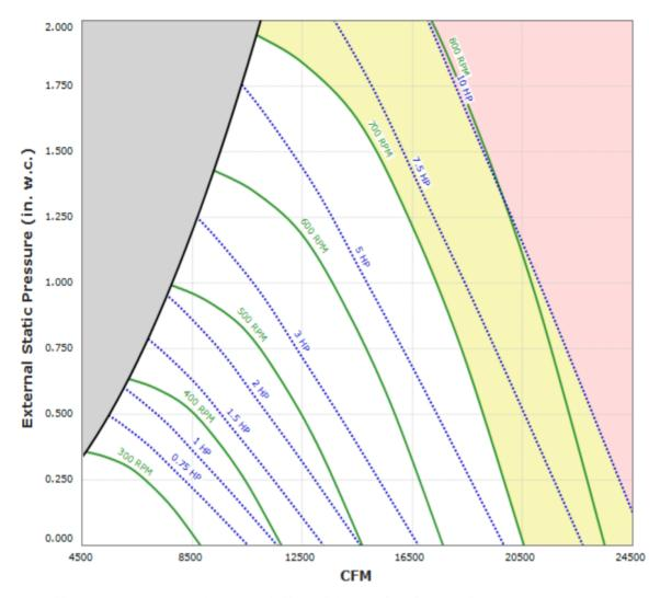
Max Sizable RPM= 850 RPM. Curve shown extended beyond this point for reference only.
