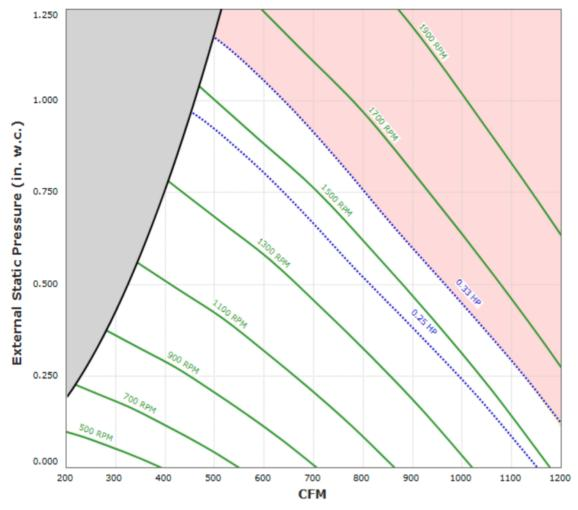
Max Sizable RPM= 2000 RPM. Curve shown extended beyond this point for reference only.
