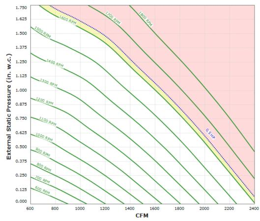
Max Sizeable RPM = 2000 RPM. Curve shown extended beyond this point for reference only.
