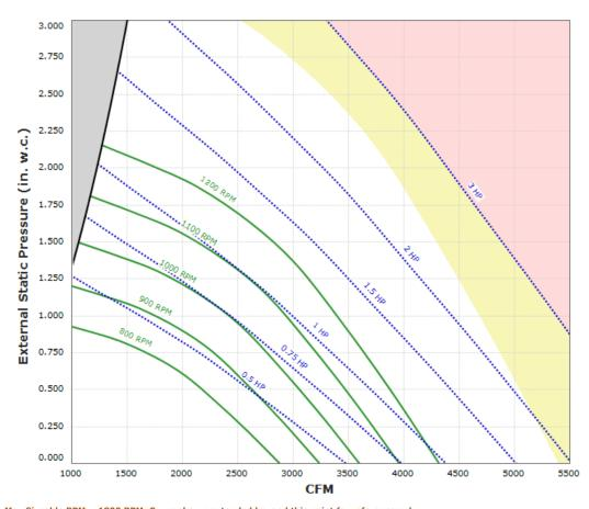
Max Sizeable RPM = 1800 RPM. Curve shown extended beyond this point for reference only. Performance shown is certified for Installation Type A: Free inlet, Free outlet. Performance ratings do not include the effects of appurtenances in the airstream. Power rating (BHP) does not include transmission losses.
