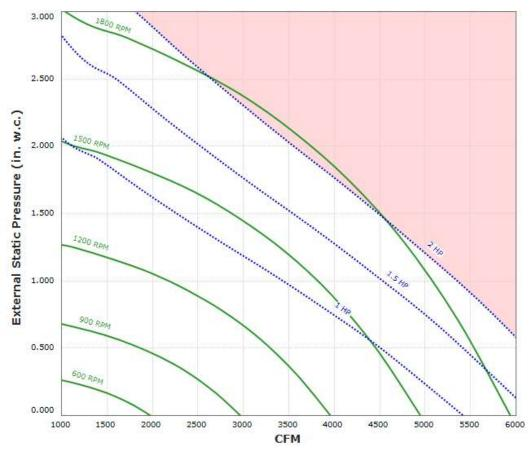
Max Sizeable RPM = 2600 RPM. Curve shown extended beyond this point for reference only.
