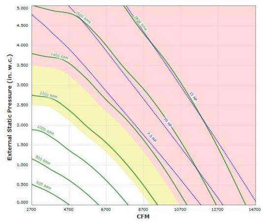
Max Sizeable RPM = 1350 RPM. Curve shown extended beyond this point for reference only.
