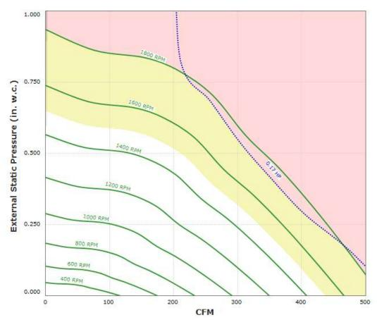
Max Sizeable RPM = 1800 RPM. Curve shown extended beyond this point for reference only.
