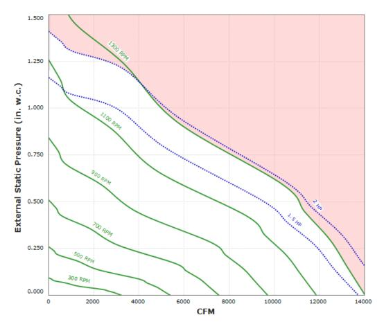
Max Sizeable RPM = 1300 RPM. Curve shown extended beyond this point for reference only.
