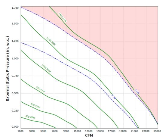
Max Sizeable RPM = 1400 RPM. Curve shown extended beyond this point for reference only.
