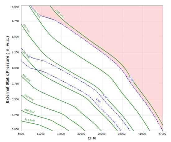
Max Sizeable RPM = 1000 RPM. Curve shown extended beyond this point for reference only.
