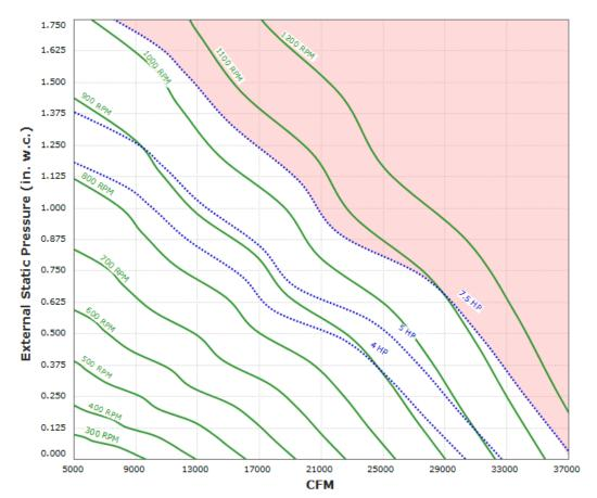
Max Sizeable RPM = 1150 RPM. Curve shown extended beyond this point for reference only.
