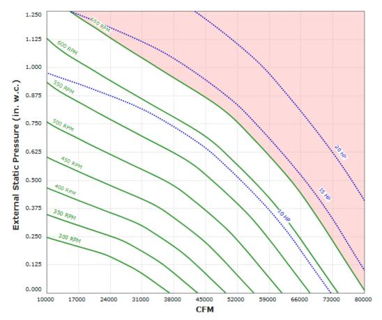
Max Sizeable RPM = 650 RPM. Curve shown extended beyond this point for reference only.
