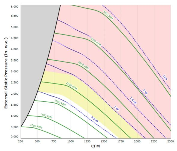
Max Sizeable RPM = 2400 RPM. Curve shown extended beyond this point for reference only. Max discharge velocity for restaurant applications is 1800 fpm. This equates to 1688 cfm.
