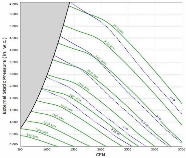
Max Sizeable RPM = 2200 RPM. Curve shown extended beyond this point for reference only. Max discharge velocity for restaurant applications is 1800 fpm. This equates to 1932 cfm.
