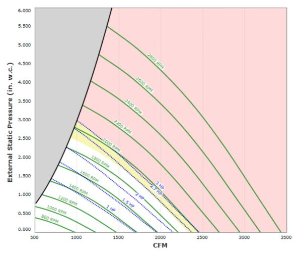
Max Sizeable RPM = 2300 RPM. Curve shown extended beyond this point for reference only. Max discharge velocity for restaurant applications is 1800 fpm. This equates to 2056 cfm.
