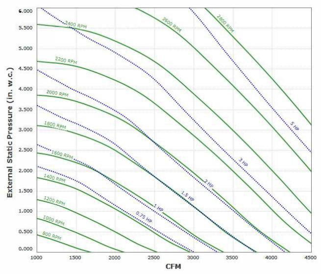
Max Sizeable RPM = 2200 RPM. Curve shown extended beyond this point for reference only. Max discharge velocity for restaurant applications is 1800 fpm. This equates to 2362 cfm.
