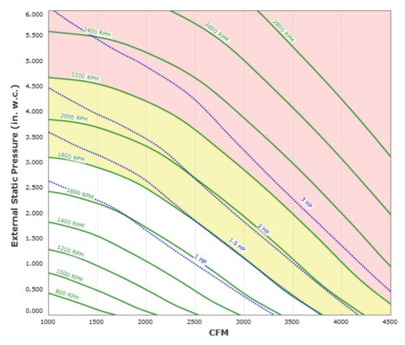
Max Sizeable RPM = 2200 RPM. Curve shown extended beyond this point for reference only. Max discharge velocity for restaurant applications is 1800 fpm. This equates to 2590 cfm.
