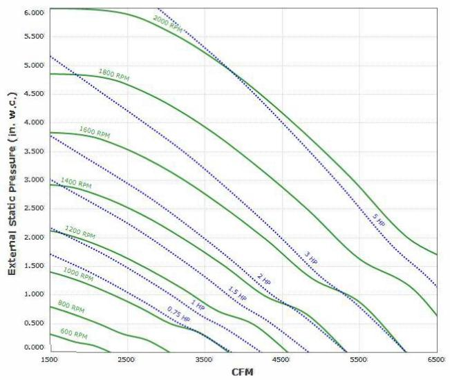
Max Sizeable RPM = 1800 RPM. Curve shown extended beyond this point for reference only. Max discharge velocity for restaurant applications is 1800 fpm. This equates to 3512 cfm.
