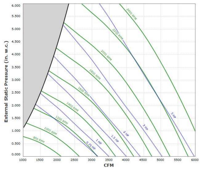
Max Sizeable RPM = 2000 RPM. Curve shown extended beyond this point for reference only. Max discharge velocity for restaurant applications is 1800 fpm. This equates to 3512 cfm.
