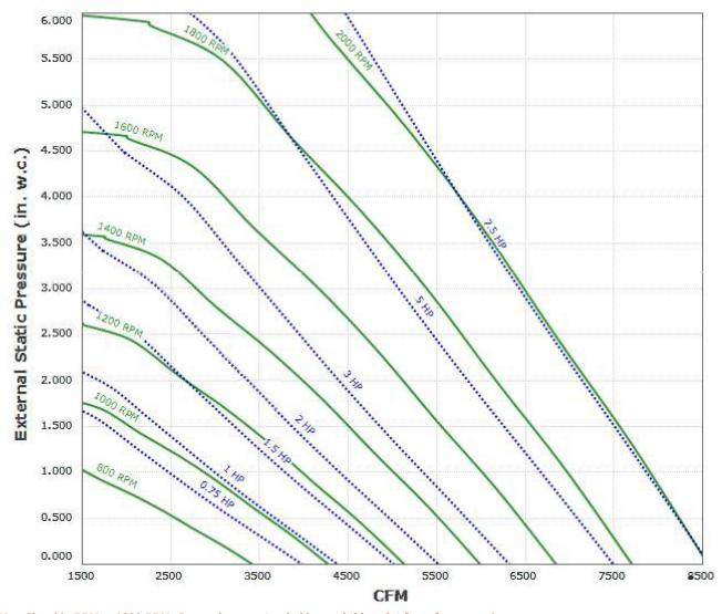
Max Sizeable RPM = 1800 RPM. Curve shown extended beyond this point for reference only. Max discharge velocity for restaurant applications is 1800 fpm. This equates to 4184 cfm.
