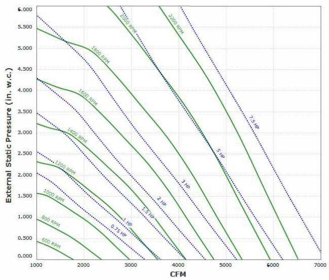
Max Sizeable RPM = 2000 RPM. Curve shown extended beyond this point for reference only. Max discharge velocity for restaurant applications is 1800 fpm. This equates to 4184 cfm.
