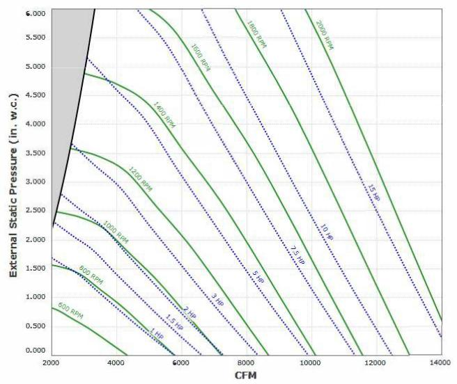
Max Sizeable RPM = 1400 RPM. Curve shown extended beyond this point for reference only. Max discharge velocity for restaurant applications is 1800 fpm. This equates to 6297 cfm.
