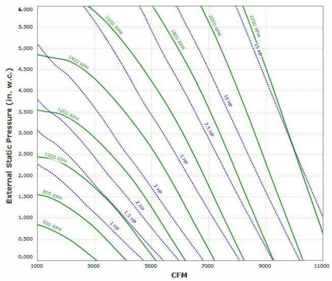
Max Sizeable RPM = 1600 RPM. Curve shown extended beyond this point for reference only. Max discharge velocity for restaurant applications is 1800 fpm. This equates to 6297 cfm.
