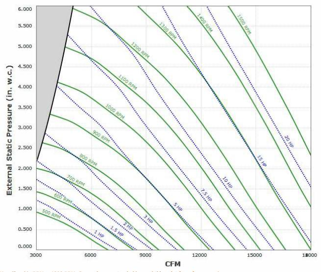
Max Sizeable RPM = 1200 RPM. Curve shown extended beyond this point for reference only. Max discharge velocity for restaurant applications is 1800 fpm. This equates to 9376 cfm.
