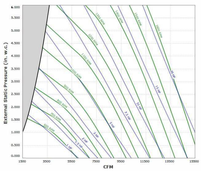
Max Sizeable RPM = 1300 RPM. Curve shown extended beyond this point for reference only. Max discharge velocity for restaurant applications is 1800 fpm. This equates to 9376 cfm.
