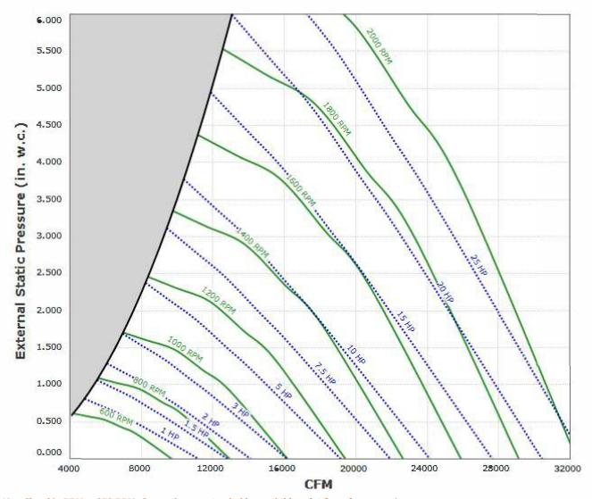
Max Sizeable RPM = 950 RPM. Curve shown extended beyond this point for reference only. Max discharge velocity for restaurant applications is 1800 fpm. This equates to 13881 cfm.
