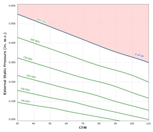
Max Sizeable RPM = 940 RPM. Curve shown extended beyond this point for reference only.
