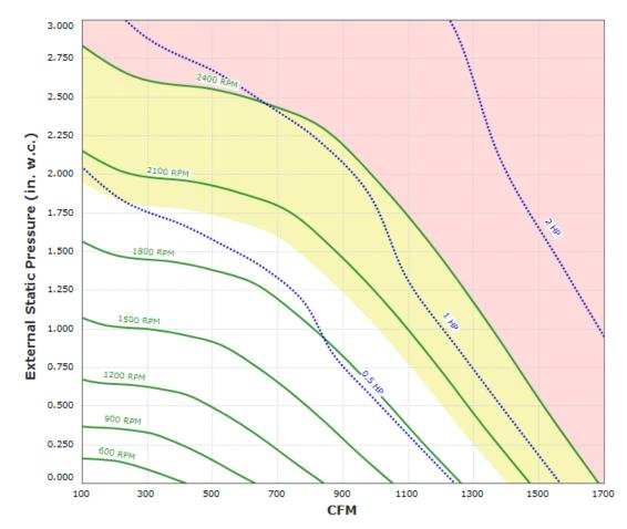
Max Sizeable RPM = 2400 RPM. Curve shown extended beyond this point for reference only. Max discharge velocity for restaurant applications is 1800 fpm. This equates to 1725 cfm.
