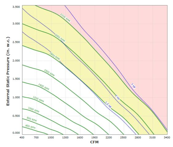
Max Sizeable RPM = 2200 RPM. Curve shown extended beyond this point for reference only. Max discharge velocity for restaurant applications is 1800 fpm. This equates to 2450 cfm.
