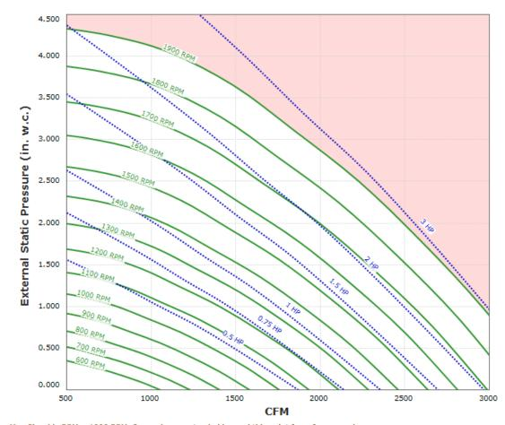
Max Sizeable RPM = 1900 RPM. Curve shown extended beyond this point for reference only. Max discharge velocity for restaurant applications is 1800 fpm. This equates to 3106 cfm.
