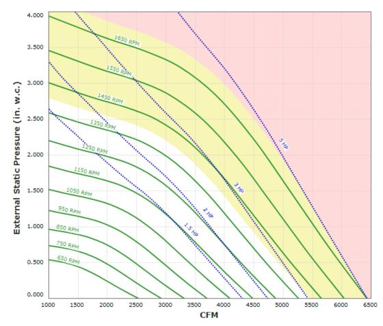
Max Sizeable RPM = 1700 RPM. Curve shown extended beyond this point for reference only. Max discharge velocity for restaurant applications is 1800 fpm. This equates to 3875 cfm.
