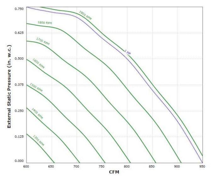
Max Sizeable RPM = 1884 RPM. Curve shown extended beyond this point for reference only. Motor M055PWCUK0315-ECM-50-115 has an rpm range of 1200 to 1800. Motor M055PWCUK0315-ECM-50-230 has an rpm range of 1200 to 1800. Motor M055PWCUK0315-ECM-60-115 has an rpm range of 1200 to 1800. Motor M055PWCUK0315-ECM-60-230 has an rpm range of 1200 to 1800.
