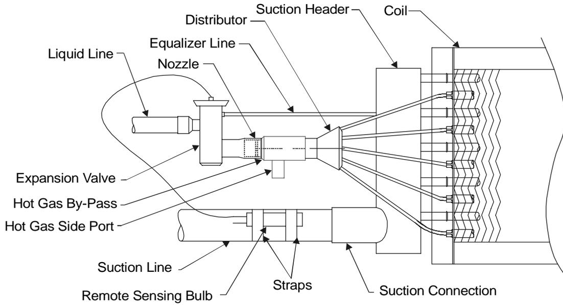
**Figure 4 - Hot Gas Bypass Kit Installed**
