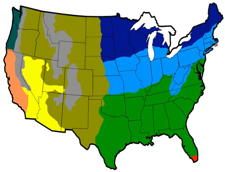
SEMIARID : 450-550 CFM/TON AND/OR EVAPORATIVE COOLING HUMID SUBTROPICAL : 360-500 CFM/TON MARINE WESTCOAST : 500-600 CFM/TON AND/OR EVAPORATIVE COOLING MEDITERRANEAN : 500-600 CFM/TON AND/OR EVAPORATIVE COOLING WARM SUMMER : 400-500 CFM/TON COOL SUMMER: 500-600 CFM/TON HIGHLAND ALPINE : 500-600 CFM/TON AND/OR EVAPORATIVE COOLING TROPICAL WET : 360-400 CFM/TON DESERT : 360-400 CFM/TON AND/OR EVAPORATIVE COOLING
