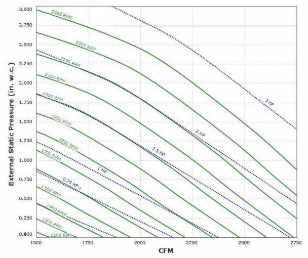
Max Sizeable RPM = 2400 RPM. Curve shown extended beyond this point for reference only.
