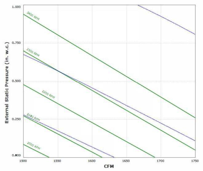
Max Sizeable RPM = 2400 RPM. Curve shown extended beyond this point for reference only.
