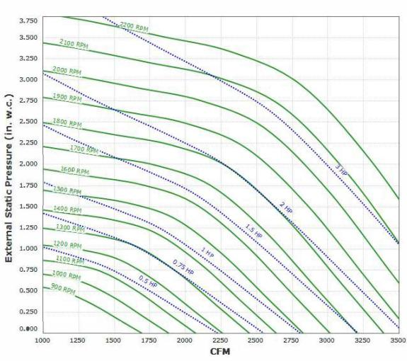
Max Sizeable RPM = 2200 RPM. Curve shown extended beyond this point for reference only.
