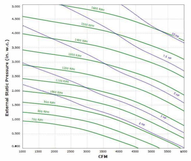
Max Sizeable RPM = 1600 RPM. Curve shown extended beyond this point for reference only.
