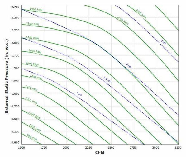
Max Sizeable RPM = 2200 RPM. Curve shown extended beyond this point for reference only.
