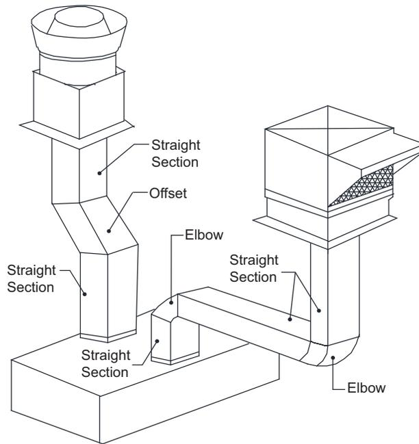
Use offsets if the duct cannot be routed straight up.
