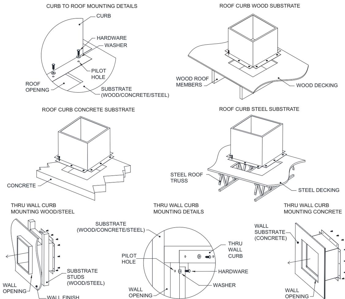
**Figure 3 - Minimum Edge Distance and Penetration Details**
