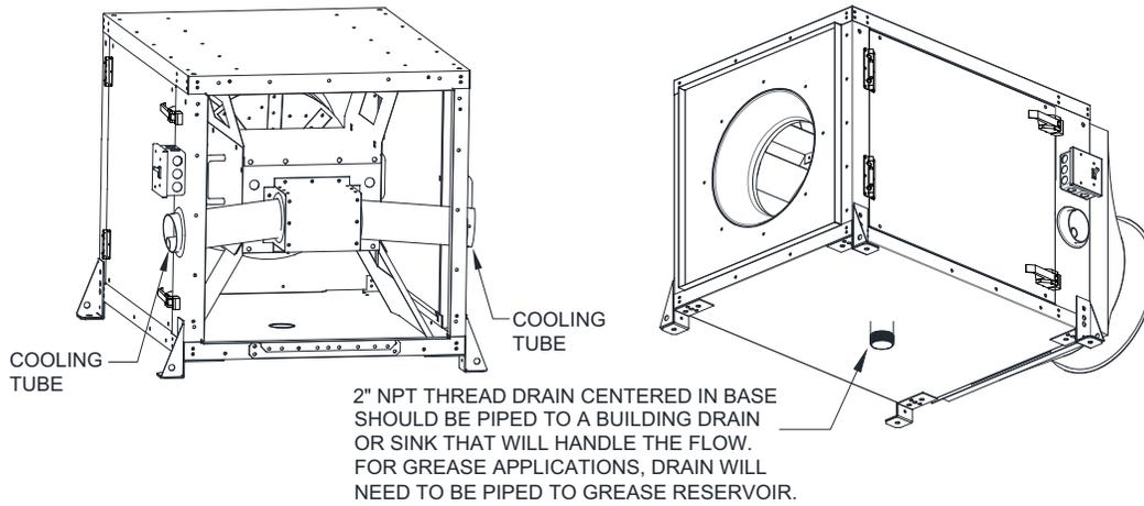
\*FAN MUST BE INSTALLED WITH DRAIN POINTING DOWN.
