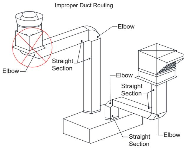
DO NOT connect elbow directly to fan inlet.
